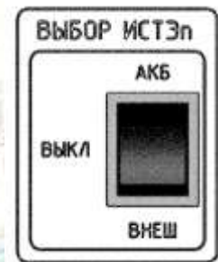
Figure 14 Power source selection switch
