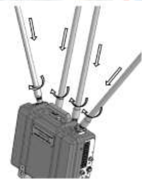
Figure 12 Installing antennas on the channel suppression unit
