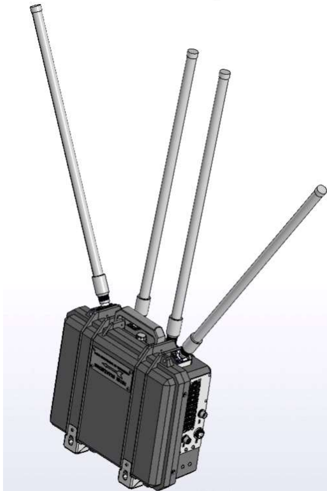
Figure 2 – Suppression Block PAKB.464514.803 with connected antennas.
