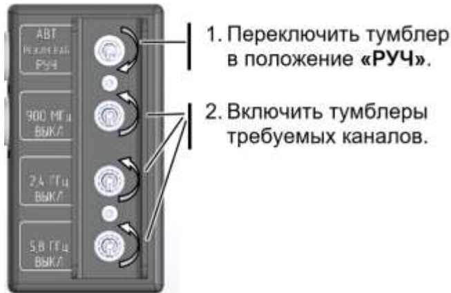
Figure 15 Controls of the product on the control panel in manual mode
