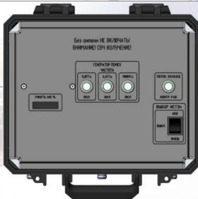
Figure 7 Control panel of the channel suppression unit
