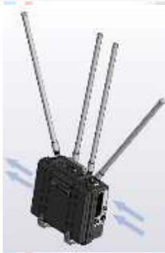
Figure 11 Product cooling flows
